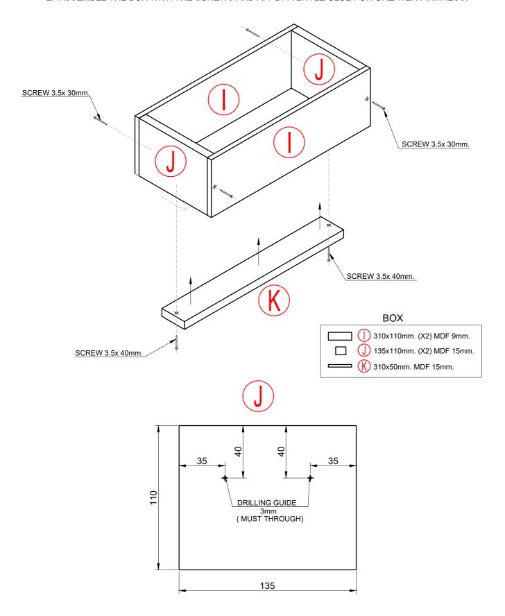
3.- JOIN BOX TO INTERNAL FACES "A" AND "B" WITH 3.5x 30mm SCREW. AND APPLY GLUE. (BE CAREFUL THAT THE SCREW DOES NOT PUNCH THE FRONT FACE OF THE DOG)
