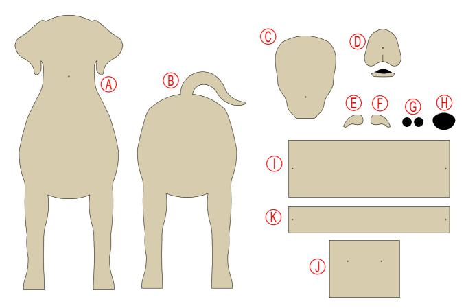
5.- JOIN PIECES "D" AND "C" TO PIECE "A" WITH A 3.5x 40mm SCREW. AND APPLY GLUE.
